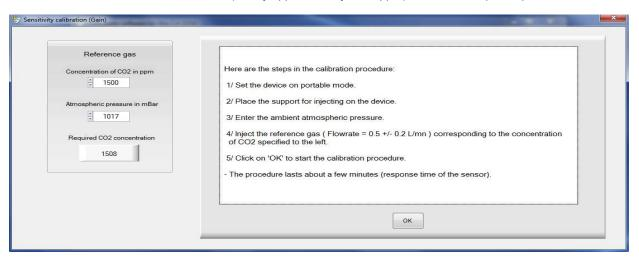
After validation, the software allows enough time for the C.A 1510 to stabilize the measurement, then acquires the measurement(s) and programs the calibration parameters.
