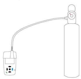
Note: The C.A 1510 must be used in portable mode in order to obtain a stable measurement as rapidly as possible. The ECO mode and recordings are prohibited for verification or calibration. The 1D and 3D modes are not recommended because they query the CO<sub>2</sub> sensor once a minute.
