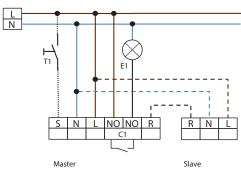
T1 = NO button for semi-automatic mode Slave for enlargement of detection area
