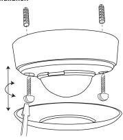
The detector must be installed on a solid and level surface. There is no need for frames.
