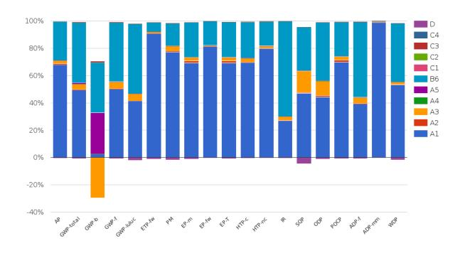
The chart shows the contribution analysis in the individual modules. It can be seen that the greatest impact on the environment is caused by the manufacturing of the luminaires and their use in the usage phase. The actual impact in B6 depends on the usage scenario, luminaire settings and the energy mix. The impact can therefore vary depending on the usage scenario.
