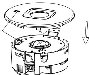
Assemble back trim plate, notice the test switch button has to align to the hole on trim plate.
