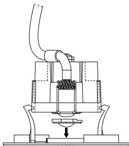
Remove current lens and replace with the other lens on trim plate.
