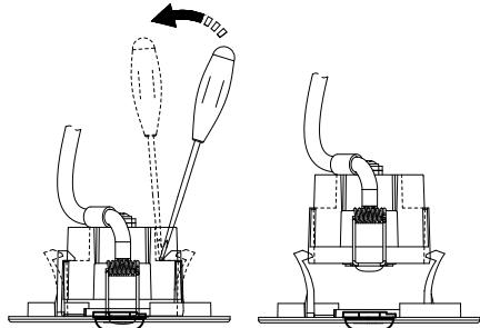
Pry off right and left bracket of trim plate, loose trim plate from heat sink, still keep trim plate snap on the heat sink.
