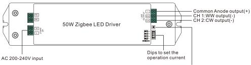
Program Key: short press to switch on/off load, press and hold down to increase/decrease light intensity
