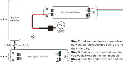
Step 2: Set another device or remote or touch panel into network pairing mode and pair to the network, refer to
