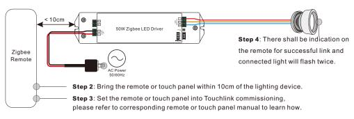
Note: 1) Directly TouchLink (both not added to a ZigBee network), each device can link with 1 remote.
