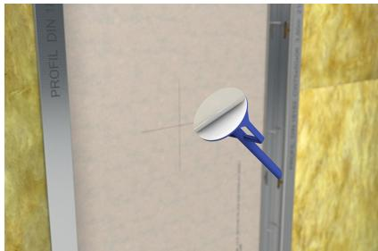
Stick the adhesive disc onto the and remove the protective film.
