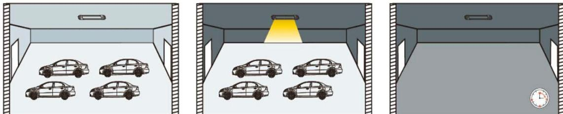
① With sufficient ambient light, the light will not be switched on.
