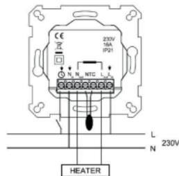
Now position the thermostat and fasten it in the wall installation box with 2 screws. Install the cover parts, fasten them with the screw and, finally, press the rotary knob in at the correct position.
