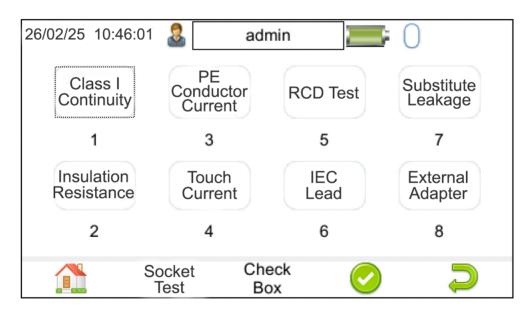
To view / edit / configure the test settings of a **Manual Test**, where appropriate, you can change the test duration, test pass / fail limit or test type / connection. Once the required
