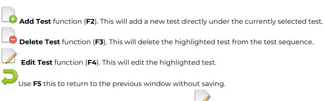
To edit the name of the sequence press the **Edit** button (**F4**). You can then give it a relevant name and press the save button to store (**F4**).
