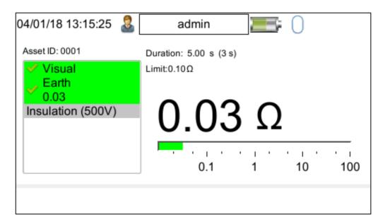
The instrument has probe detection that will automatically flag up if you do not have the correct probe configuration for the test you are trying to perform.
