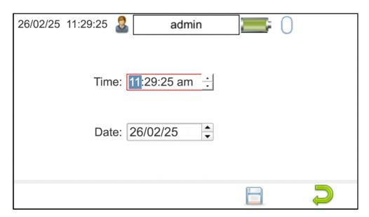
Use the left/right keyboard arrow keys to highlight the required parameter and then use the up/down keyboard keys to increase or decrease this, respectively.
