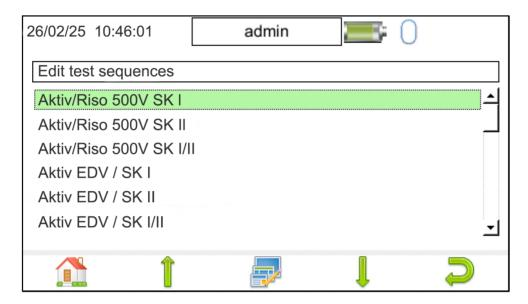
Altering **Test Sequences**: with a sequence highlighted, press the menu button open the **Test Sequence Options** menu.
