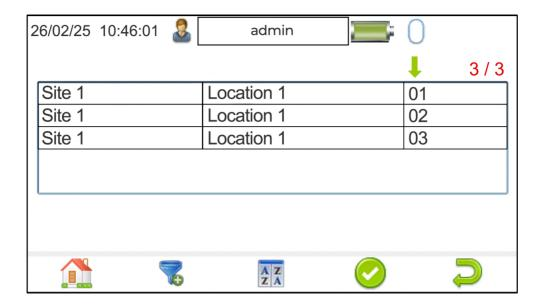
This is the **Accept** function, use the keyboard arrow keys to highlight an asset and use **F4** view any corresponding results.
