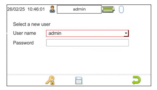
Use this button (F2 in the Select a new user window) to change the password for the current user. Enter the Existing Password, enter a New Password and then Confirm New Password.
