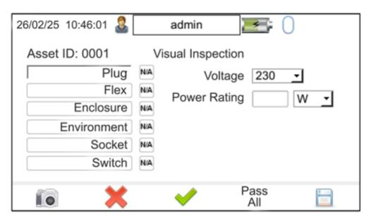
Using the Camera in this screen (F1) will tag the picture to the test result.
