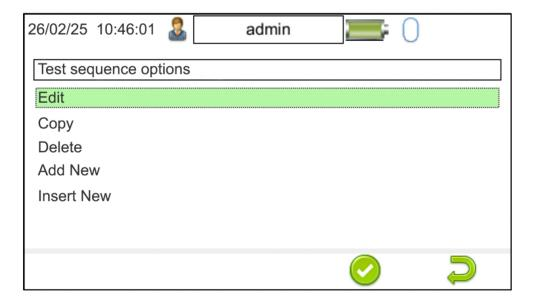
Select **Add New** using the keyboard arrow keys and the **Accept** button (F4). This will add a **New Test Sequence** to the bottom of the test sequence list.
