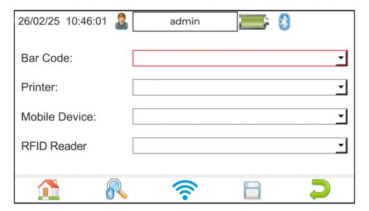
The **Bluetooth® Search** button (**F2**) will search the area for Bluetooth® discoverable devices (= Bluetooth® is turned on) and return to the previous menu. You can then use the keyboard arrow keys to select the correct Bluetooth® ID from the dropdowns:
