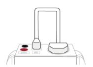
The Polarity test checks the wiring polarity of an IEC lead, the IEC should be plugged into both the EUT socket and IEC test sockets on the instrument.
