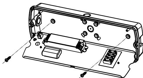
Install fixture on mounting surface by screws.
