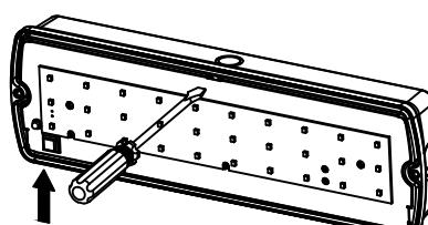
Use blade screwdriver insert the slot and pry off the steel plate.
