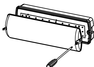
Remove screws by screwdriver then remove the cover.
